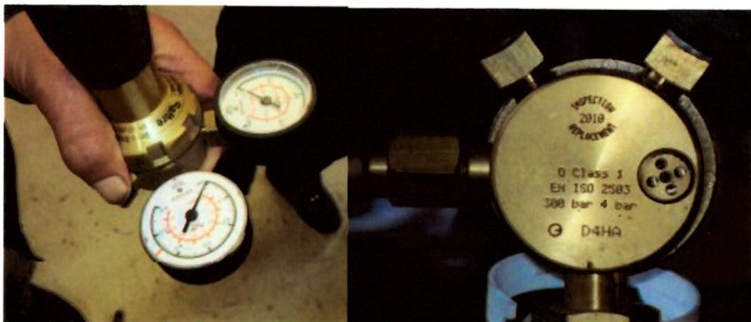
5.5.1 Figure 4: Damaged regulator and information plate
